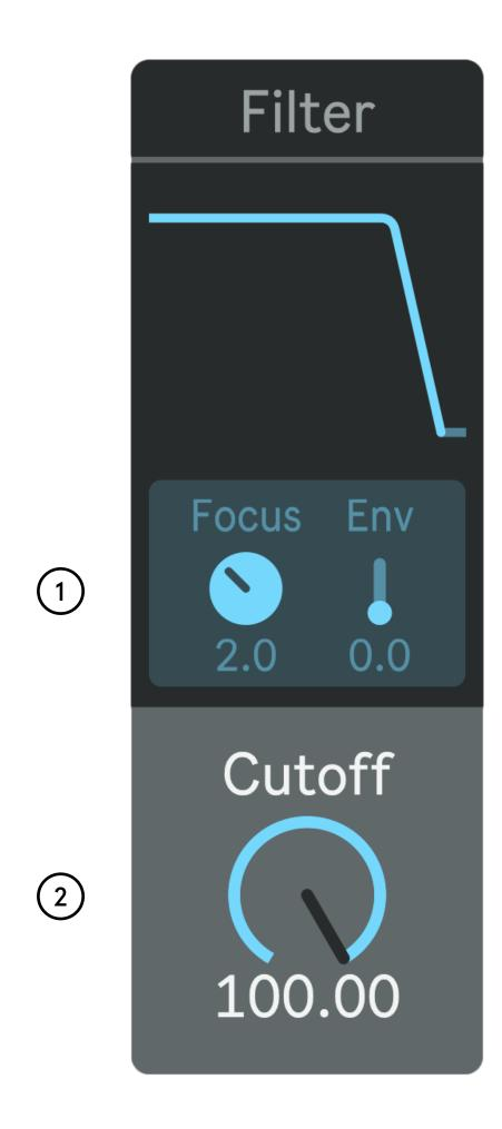
The Filter is a non-resonant lowpass filter with dynamic mixing between filter poles for variable steepness.
