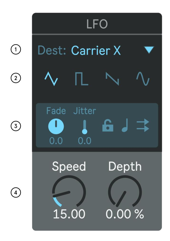
The LFO is a Low Frequency Oscillator that can introduce movement to various parameters.
